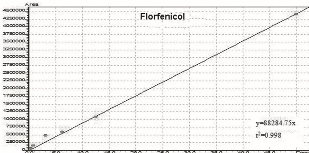
**Figure 1.** The standard curve of the concentrations of florfenicol prepared using peak areas obtained in HPLC.
