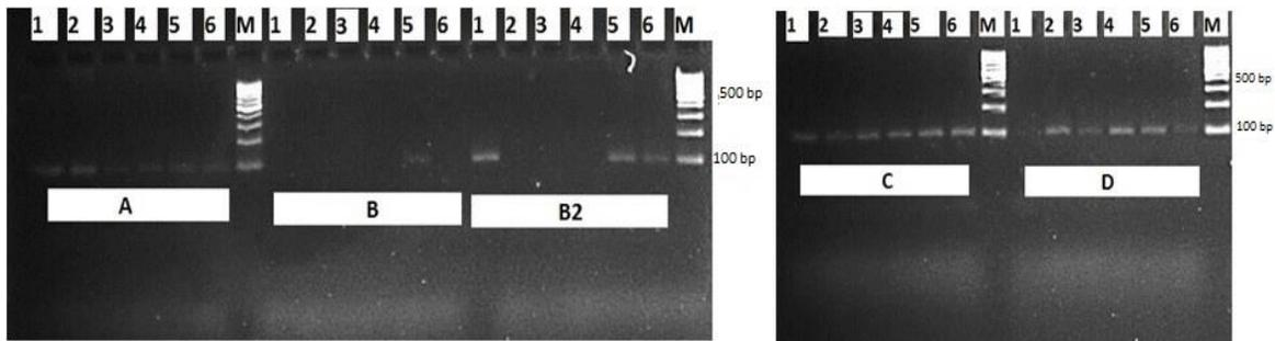
**Figure 2. Results of PCR.** A: DNA isolation kit, B: DTAB method (100 mg), B2: DTAB method (20 mg), C: CTAB method, D: Phenol / chloroform method, 1) Meatball, 2) Salami, 3) Sucuk, 4) Braised meat, 5) Sausage, 6) Pastrami, M: Molecular marker (100 bp)
